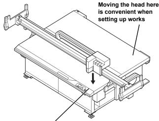
Moving the head here is convenient when mounting tools
