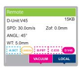
SPD: Cutting speed Zof: Z origin offset value ANGL: Edge angle WT: Work thickness
