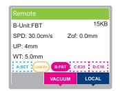
SPD: Cutting speed Zof: Z origin offset value UP: Up height WT: Work thickness
