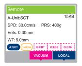
SPD: Cutting speed PRS: Cutting pressure Eofs: Offset value WT: Work thickness
