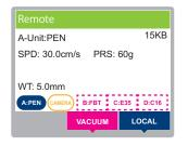
SPD: Cutting speed PRS: Cutting pressure WT: Work thickness
