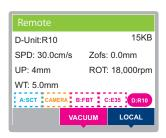
SPD: Cutting speed Zof: Z origin offset value UP: Up height ROT: Rpm WT: Work thickness
