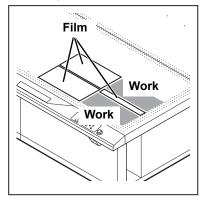
When a work is positioned away from the work guide
