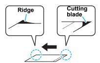
• When mounting an NT high-speed steel blade, use the hand lapper provided to grind down the cutting edge and ridge.
