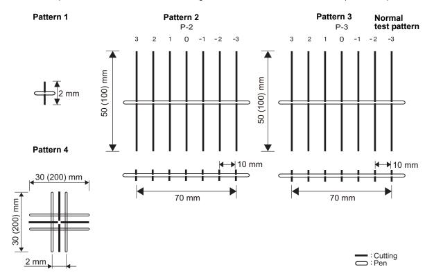
Adjust using the four theta angle adjustment patterns in sequence from pattern 1. Adjust in the sequence Pattern  $1 \rightarrow$  Pattern  $2 \rightarrow$  Pattern 3 to achieve increasingly fine angle adjustment. (Pattern 4 is used to check the adjustment.)
