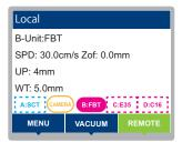
Press (a) (c) to select [Setup] > [Command] > [OH: Response Value], then press the [ENTER] key.
