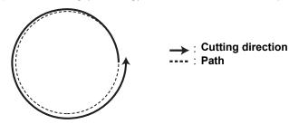
Values of circle θ correction are automatically calculated based on the radius of circles to draw.
