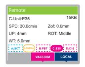
SPD: Cutting speed Zof: Z origin offset value UP: Up height ROT: Reciprocating vibration level WT: Work thickness
